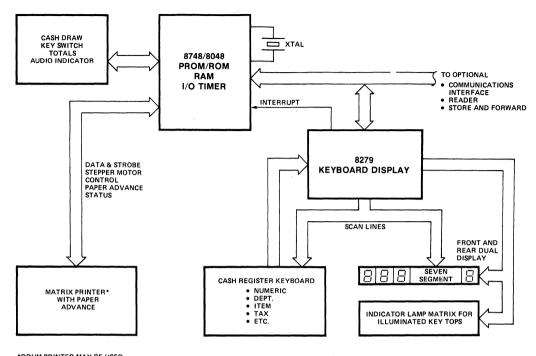
\*DRUM PRINTER MAY BE USED. DRUM PRINTER REQUIRES MORE OUTPUTS WHICH CAN BE OBTAINED FROM AN EXPANDER DEVICE.
